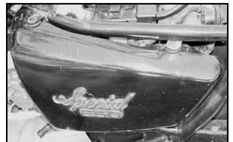
All 1980-84 (except 80G) Type Grommet mount damper rubbers used on upper & lower mount points.
