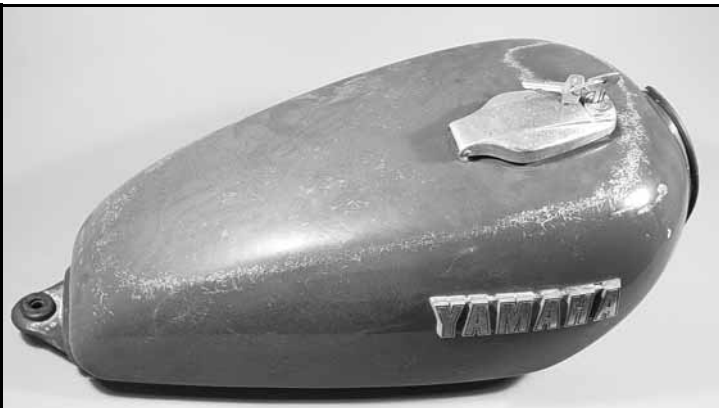
Gas Tank - 1977-84 "Specials" Offset locking gas cap, 2 vacuum type petcocks on -
