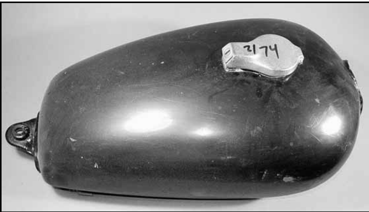
Gas Tank - 1974-75 Locking Cap (Key at rear) with cap in center of tank, 2 manual petcocks
