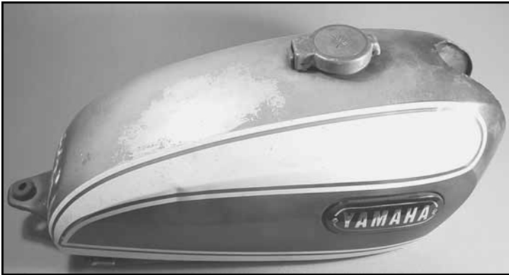
Gas Tank - Fits: 1970-73 Models Only. Non Locking Cap in center of tank, 2 manual petcocks
